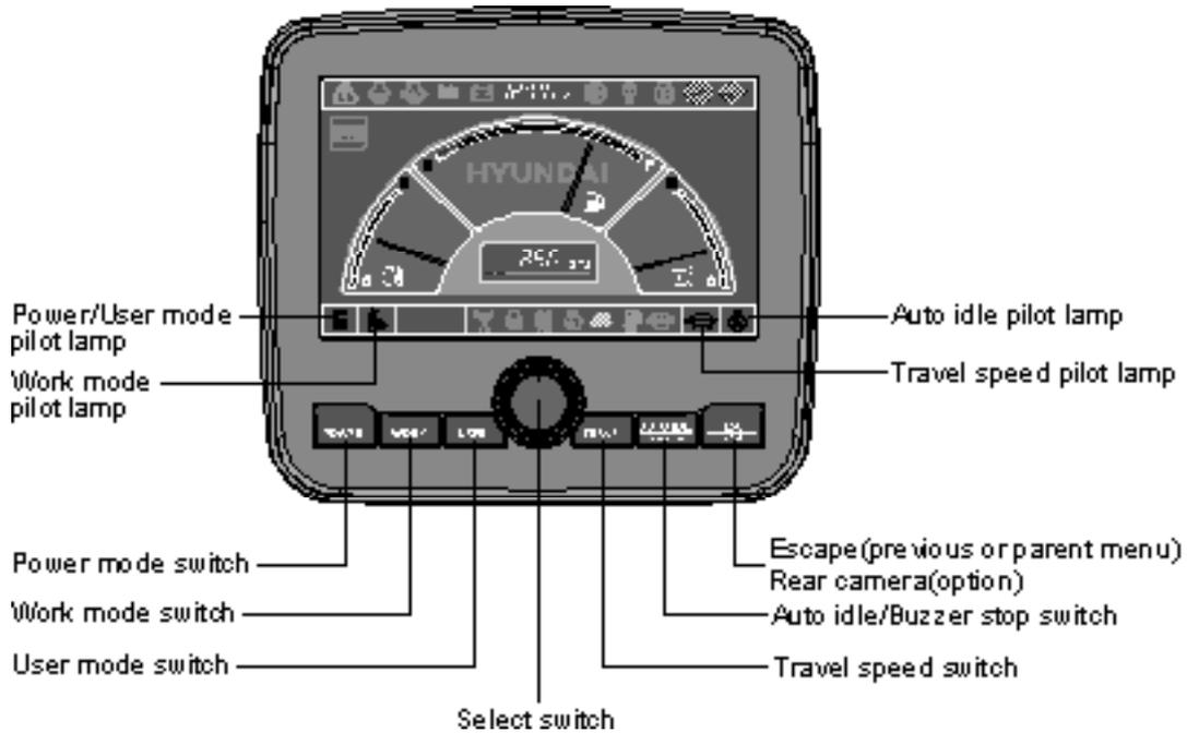
※ When the switches are selected, the pilot lamps are displayed on the LCD. Refer to the page 3-7 for details.
