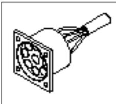
(1) MCU communicates the machine data with Laptop computer through RS232 service socket.
